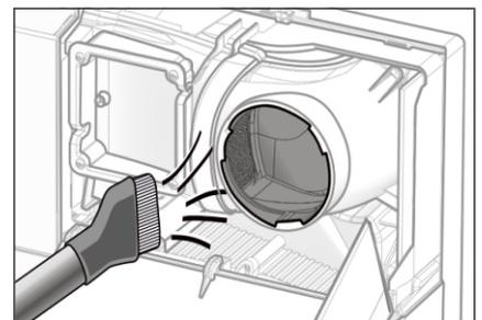
6. Remove dirt from both ducts with a vacuum cleaner or a soft cloth (do not use water).
