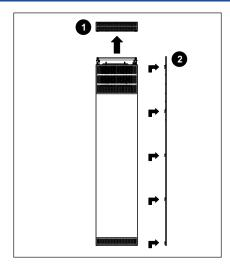
1. First remove the top grid of the unit (1). Then the right side panel (2). This is where the internal control panel is attached.
