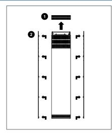
1. First remove the top grid of the appliance (1). Then the right and left side panels (2). The internal control panel is attached on the right side.
