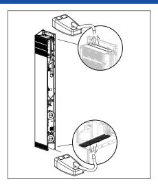
3. Clean the insect mesh at the top and bottom of the unit using your vacuum cleaner.
