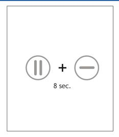
2. Set your device to service mode by holding the key combination above for 8 seconds. All LEDs will light up. Wait 1 minute for the valves to close.
