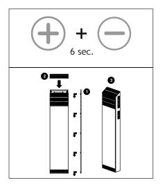
6. Reset the filter hours counter by pressing the above key combination for 6 seconds. The "filter dirty" message disappears.
