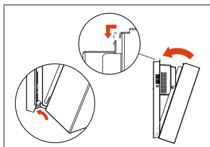
8. Place the housing by putting it in the wall frame and tilting it forward. Now lift the housing slightly so that it falls over the wall frame. Make sure that the cabling is not jammed anywhere. *If applicable, replace the locking screws.*
