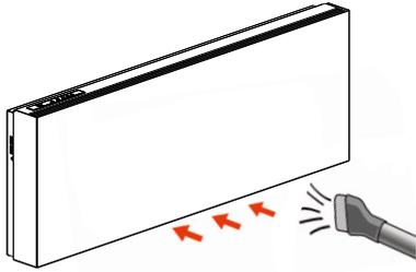
The exhaust air filters are located at the bottom of the device.
