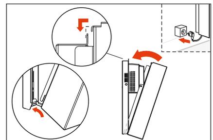
9. Place the housing by putting it in the wall frame and tilting it forward. Now lift the housing slightly so that it falls over the wall frame. Make sure that the cabling is not jammed anywhere. Plug it in. *Replace, if applicable, the locking screws.*
