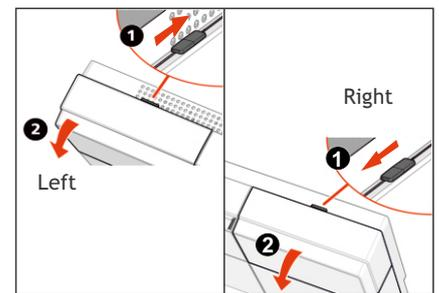
3. Push the left and right locking slide on top of the ClimaRad ventilation unit inwards and open both flaps by pulling them towards you.
