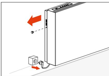
1. First, turn off the device by unplugging it from the power outlet. Then (if any) remove the locking screws on both sides of the wall frame.
