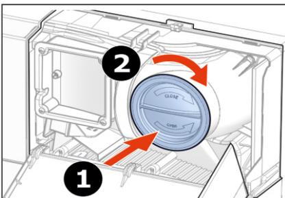
7. Push the two blue filter caps back in completely for correct operation and tighten them.
