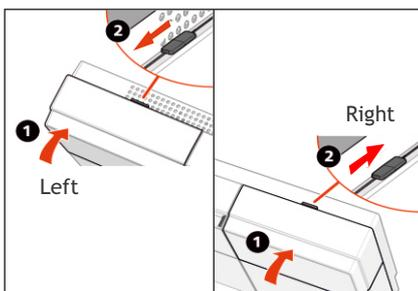
7. Close the flaps on the left and right side of the device and slide both locking sliders back.
