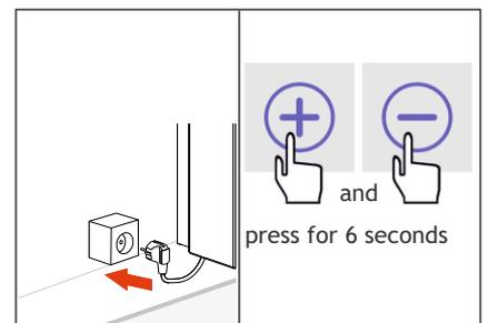
9. Plug it back in and reset the filter hour counter (press + and - simultaneously for 6 seconds). The message "filter contaminated" now disappears. **Important: Reset the filter hour counter only if you have replaced the filters.**
