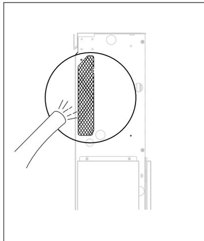
5. Clean the insect mesh on both sides of the convector using your vacuum cleaner.
