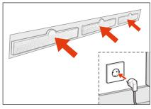
3. Push 3 new filters into the holders and then push the plug back into the socket.
