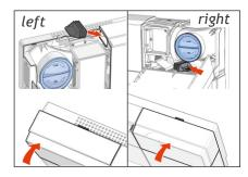
7. Put the two black filter caps (left and right) back in position and close both valves again.
