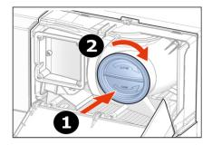
7. Push both blue filter caps back in completely in order to ensure correct operation and screw them back into position.
