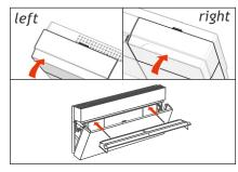
8. Close the valves and re-install the air distributor.
