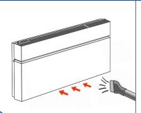
The air output filters are located at the bottom of the device. Vacuum the visible dirt off the filters. This guarantees the air flow. You do not need to remove the air output filters to do this.
