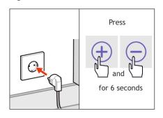
9. Put the plug back into the socket and reset the filter hour counter (Press + and - simultaneously for 6 seconds). The 'filter vervuild' message will now disappear.
