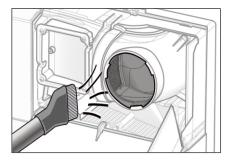
6. Remove dirt from both ducts with a vacuum cleaner or a soft cloth (do not use water).
