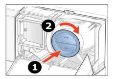
7. Push both blue filter caps fully back in for a correct operation and tighten.
