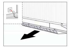
1. Pull the plug from the socket and pull the filter tray at the bottom of the ClimaRad forwards.
