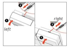
8. Close the covers on the lefthand and right-hand side of the unit, and slide both latching slides outwards.
