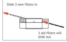
6. Slide the three new filters in the unit from the left-hand side. The old filters will automatically slide out on the right-hand side.
