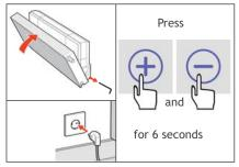
9. Unlock the radiator and tilt it back. Push the plug back into the socket and reset the filter hour counter (by simultaneously pressing on the + and - on the display for 6 seconds ). The message 'Filter vervuild' will disappear. Tighten the locking screws again.
