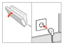
9. Unlock the radiator and tilt it back. Push the plug back into the socket and tighten the retaining screws.
