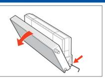
3. Tilt the radiator and, if required, lock it with an Allen key or screwdriver.
