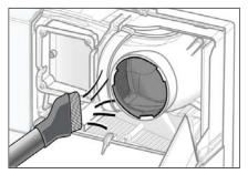
6. Remove any dirt from both channels with a vacuum cleaner or a soft cloth (do not use water).
