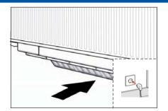
4. Slide the filter tray closed until you hear a clicking sound. Push the plug back into the socket.
