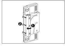
5. Tilt the filter housing back and secure with the three clips.
