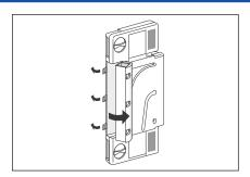
3. Open the three clips at the left-hand side of the unit and tilt the filter housing forwards
