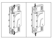
4. Slide the two dirty filters out of the filter housing and slide the two new filters fully into the filter housing.
