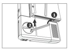
4. Insert first the right-hand side of the new filter in the outlet opening. Then push the left-hand side of the filter in the opening.
