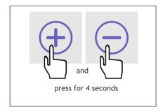
8. Reset the filter hour counter by simultaneously pressing on the + and - on the display for 4 seconds. The message 'Filter vervuild' will disappear.
