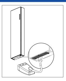
2. Clean the insect mesh at the bottom of the unit using your vacuum cleaner.
