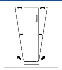
2. Remove the two screws on the top panel. Then remove one of the two side panels of the device.
