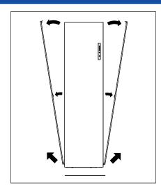
3. Remove the two screws on the top panel. Then remove one of the two side panels of the device.
