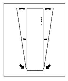
5. Place the side panel back. Than replace the two screws on the top panel.
