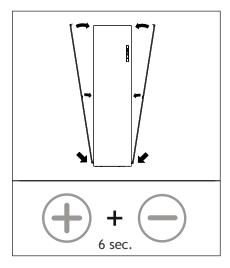
6. Place the side panel back. Than replace the two screws on the top panel. Reset the filter hour counter by holding the key combination above for 6 seconds. The "filter vervuild" notification will disappear.
