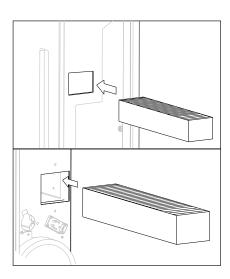
4. Remove both polluted filters and place the new inlet filter (below) and output filter (above).
