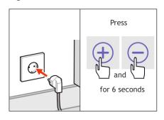
9. Put the plug back into the socket and reset the filter hour counter (Press + and - simultaneously for 6 seconds). The 'filter vervuild' message will now disappear.
