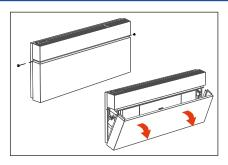
2. Unscrew the locking screws from the housing. The lower housing now moves forward.
