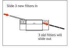
6. Slide three new filter elements into the device on the left side. The old filter elements are automatically ejected from the right side.
