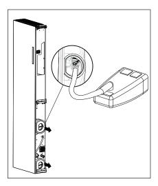
4. Remove the caps from both air ducts. Clean the duct entrances with a dry cloth or your vacuum cleaner. Also clean the insect mesh in the upper air duct. Place the caps back in the device.
