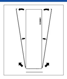
3. Remove one of the two side panels of the device.
