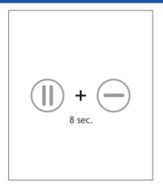
1. Set your device to service mode by holding the key combination above for 8 seconds. All LEDs will light up. Wait 1 minute for the valves to close.
