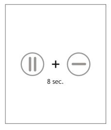
1. Set your device to service mode by holding the key combination above for 8 seconds. All LEDs will light up. Wait 1 minute for the valves to open.
