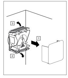
6. Remove the casing of the unit in the external room and then the two slat grilles. Clean the unit with a dry cloth or your vacuum cleaner. Place the slats and the casing back.
