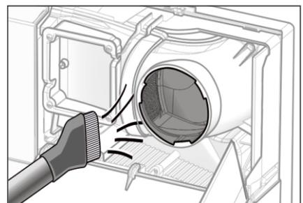
6. Remove any dirt from both channels with a vacuum cleaner or a soft cloth (do not use water).
