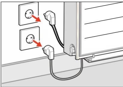
1. Switch off the device first by removing the plug from the sockets.
