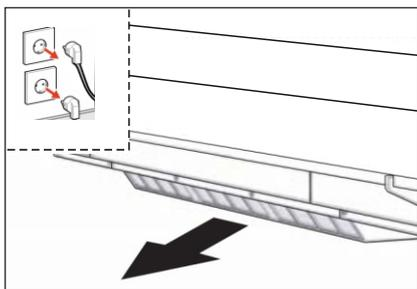
1. Remove the plug for the ventilation unit and the plug for the electrical radiator from the sockets and pull the filter tray at the bottom of the ClimaRad
