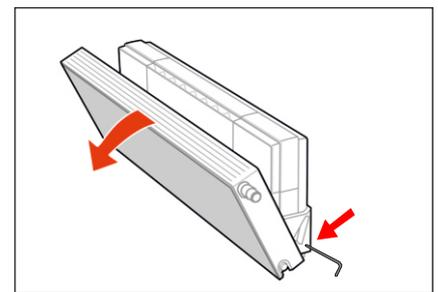
3. Tilt the radiator and, if required, lock it with an Allen key or screwdriver.
