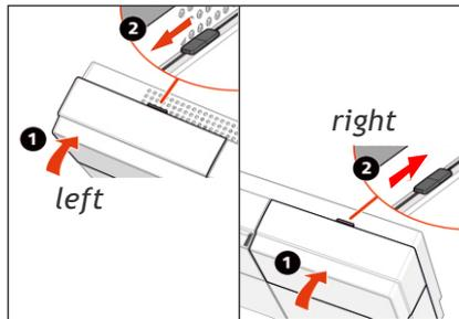
8. Close the covers on the left-hand and right-hand side of the unit, and slide both latching slides outwards.
