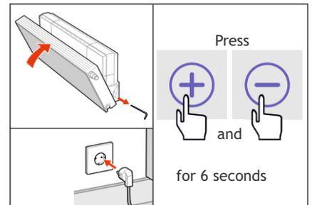
9. Unlock the radiator and tilt it back. Push the plug back into the socket and reset the filter hour counter (by simultaneously pressing on the + and - on the display for 6 seconds). The message 'Filter vervuild' will disappear. Tighten the locking screws again.
