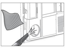
11. Remove any dirt from both channels with a vacuum cleaner or a soft cloth (do not use water).
