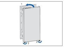
13. Put the cover back on and turn the locking hooks (at the bottom or on the side of the housing).
