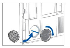
12. Insert the round cups.. Install both inspection hatches and tighten them well for a correct operation.
