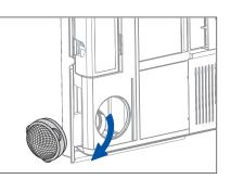
10. Remove the round cups from the air duct and remove the dust and dirt from the insect mesh.
