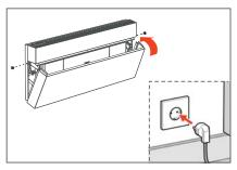
9. Tilt the lower housing back and tighten the screws again. Then put the plug back into the socket.
