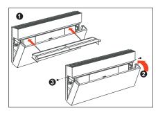
8. Reinstall the air distributor (1), tilt the lower housing back in position (2), and tighten the screws again (3).
