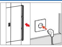
4. Slide the filter tray closed until you hear a clicking sound. Push the plug back into the socket.
