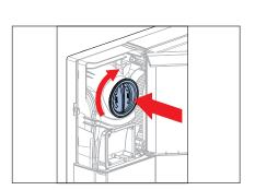
6. Push both blue filter caps fully back in for a correct operation and tighten.
