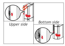
7. Close the covers on the upper and bottom side of the unit, and slide both latching slides outwards.
