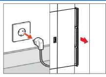
1. Pull the plug from the socket and pull the filter tray at the right side of the ClimaRad forwards.
