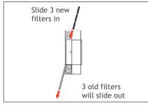
5. Slide the three new filters in the unit from the upper side. The old filters will automatically slide out on the bottom side.
