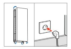
8. Put the cover back on and turn the locking hooks (at the bottom or on the side of the housing). Push the plug back into the socket.
