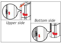
7. Close the covers on the upper and bottom side of the unit, and slide both latching slides outwards.
