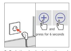
9. Push the plug back into the socket and reset the filter hour counter (by simultaneously pressing on the + and - on the display for 6 seconds ). The message 'Filter vervuild' will disappear. Tighten the locking screws again.
