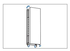
8. Put the cover back on and turn the locking hooks (at the bottom or on the side of the housing).
