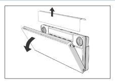
3. Tilt the radiator as far forward as possible and remove the cover.
