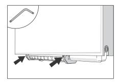
2. Turn the two locking pins outwards with an Allen key.
