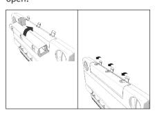
7. Tilt the filter housing close and secure with the three clips.
