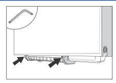
2. Turn the two locking pins outwards with an Allen key (not included).
