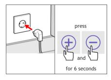
9. Push the plug back into the socket and reset the filter hour counter by simultaneously pressing on the + and - on the display for 6 seconds. The message 'Filter vervuild' will disappear.
