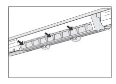
5. Place the three new filters in the sections.
