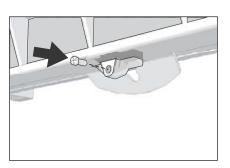
7. Screw the grille in position with the two screws.
