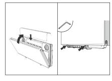
9. Install the cover and close the radiator. Then turn the two retaining pins inwards with an Allen key.
