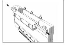
5. Slide the two contaminated filters to the left and the right out of the filter housing.
