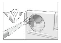
6. Remove the dirt from both channels with a vacuum cleaner or a soft cloth (do not use water).
