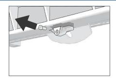
2. Loosen the two screws under the filter cover.
