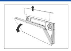
3. Tilt the radiator as far forward as possible and remove the cover.
