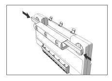
6. Slide the two new filters fully into the filter housing so that they do not project.
